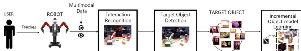
Figure 1: Overview of our approach. A human user teaches a robot new objects through natural interactions (e.g., pointing to it). The robot recognizes the type of interaction, finds the corresponding object region on its camera views and updates the object model incrementally with that data.
